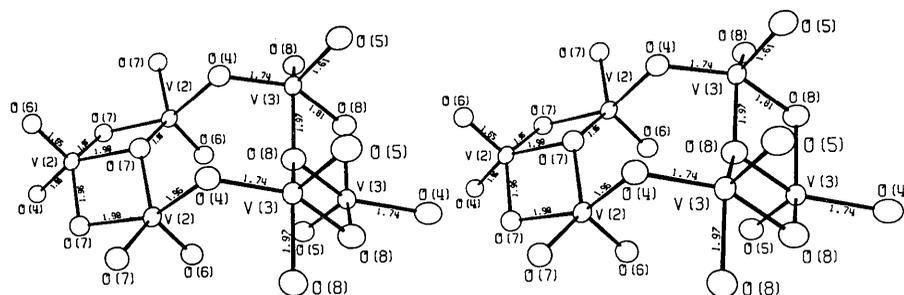
Fig. 1. A portion of the structure of  $\text{LiV}_2\text{O}_6$ , showing the coordination about the vanadium atoms.
